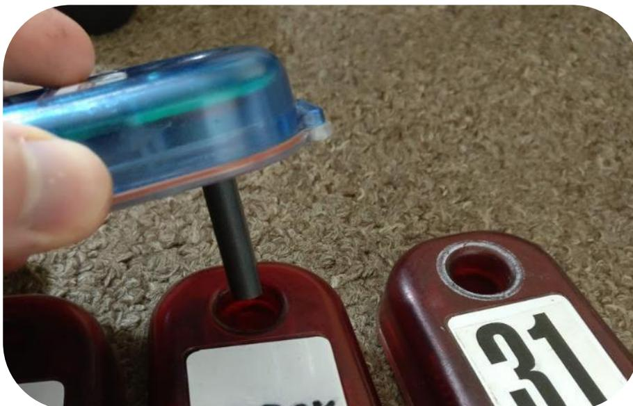
3. The Si-Master station beeps and flashes after a few seconds to show the process is complete.
